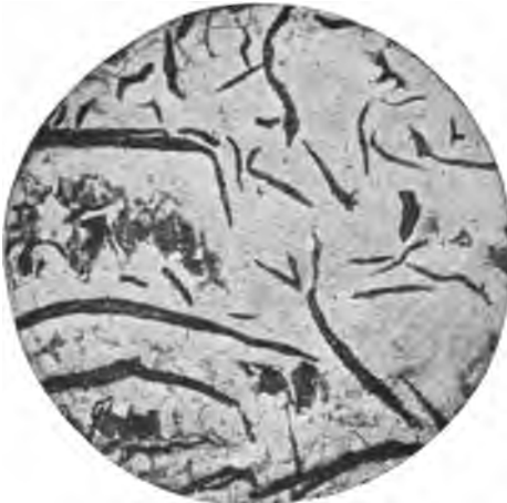
FIG. 44. — Gray Cast Iron. Magnified 100 Diameters. (Boylston.)
